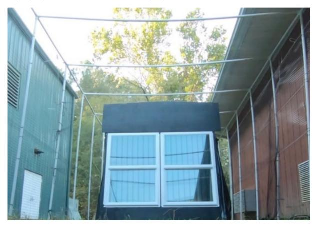
2. Study Image: Swaddle, John.2022.birdstriketest.moviestill.jpeg (jpeg attached) Caption: The daylit test arena, showing two windows with vertical lines of Haverkamp film that birds fly toward. There is a fine mist net in front of the windows to prevent actual collision.
